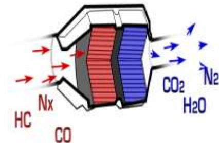
Fig.2 Basic Conversion of Catalytic Converter
